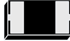
DFN1006-2L (Bottom View)
